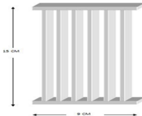
**Figure 3** Typical drawing of permeable spur model
