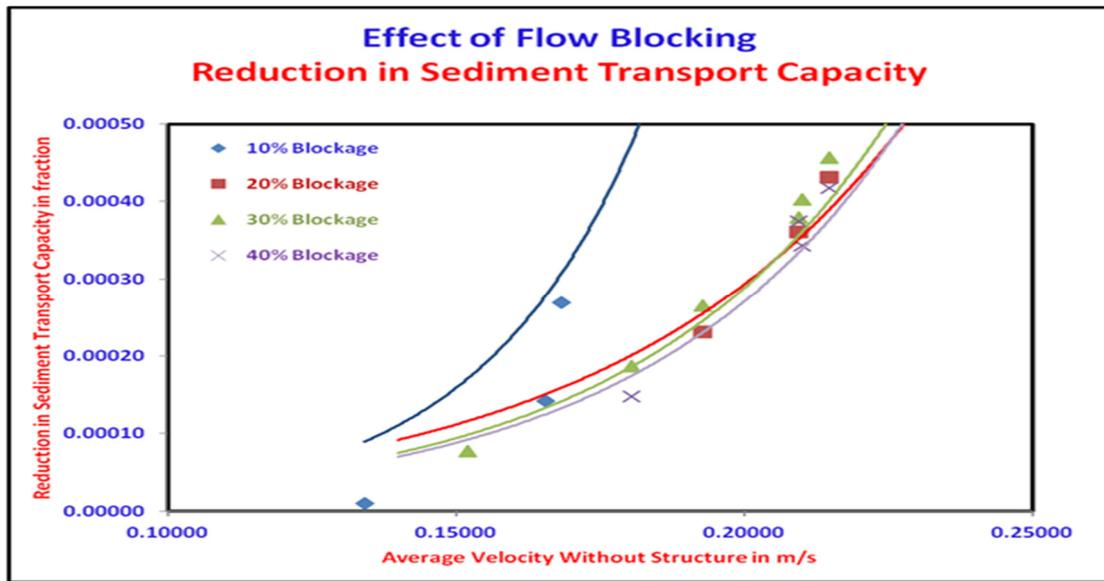
Figure 5 Graph shows effect reduction in sediment transport capacity
