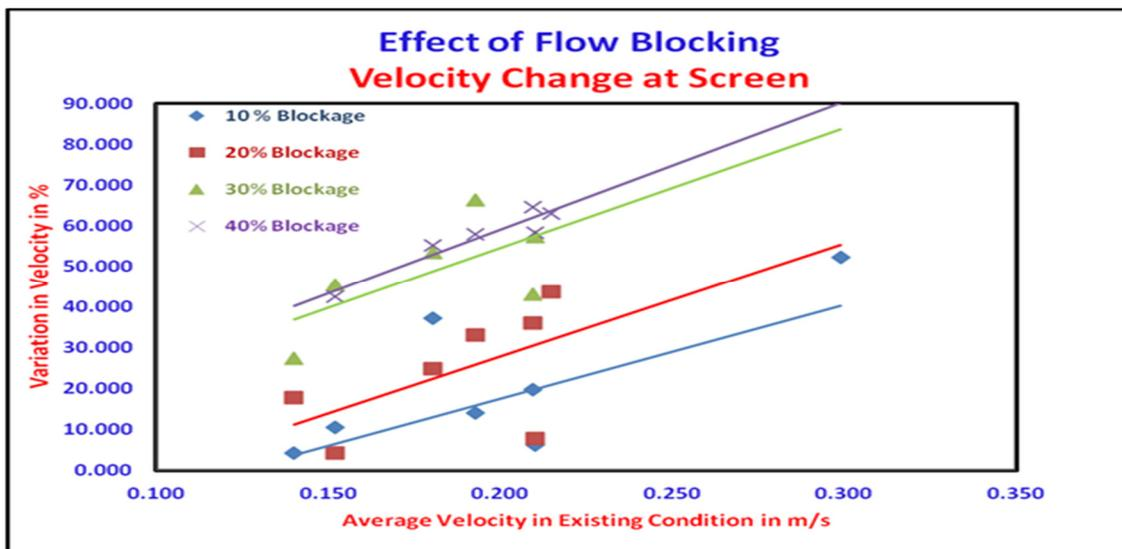
Figure 3 Graph Showing Effect of Flow Blocking due to velocity variation
