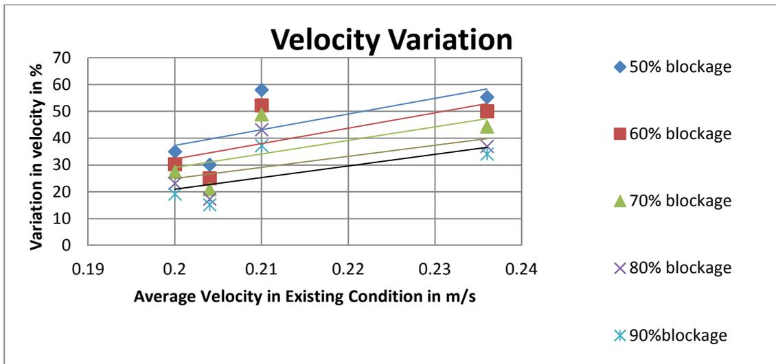
**Figure 4** Graph Showing Effect of Flow Blocking due to velocity variation
