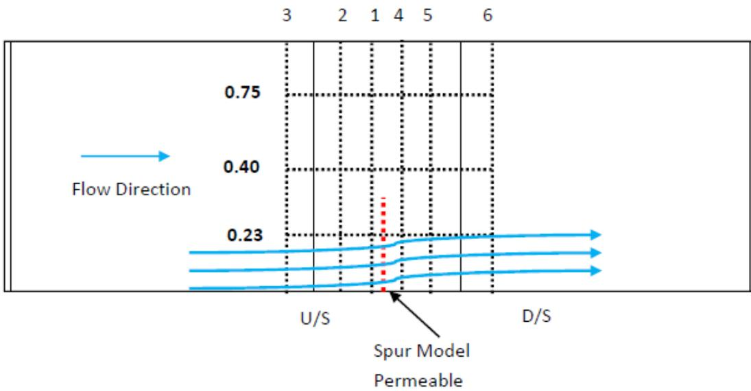
**Figure 2** layout of permeable model and flow condition
