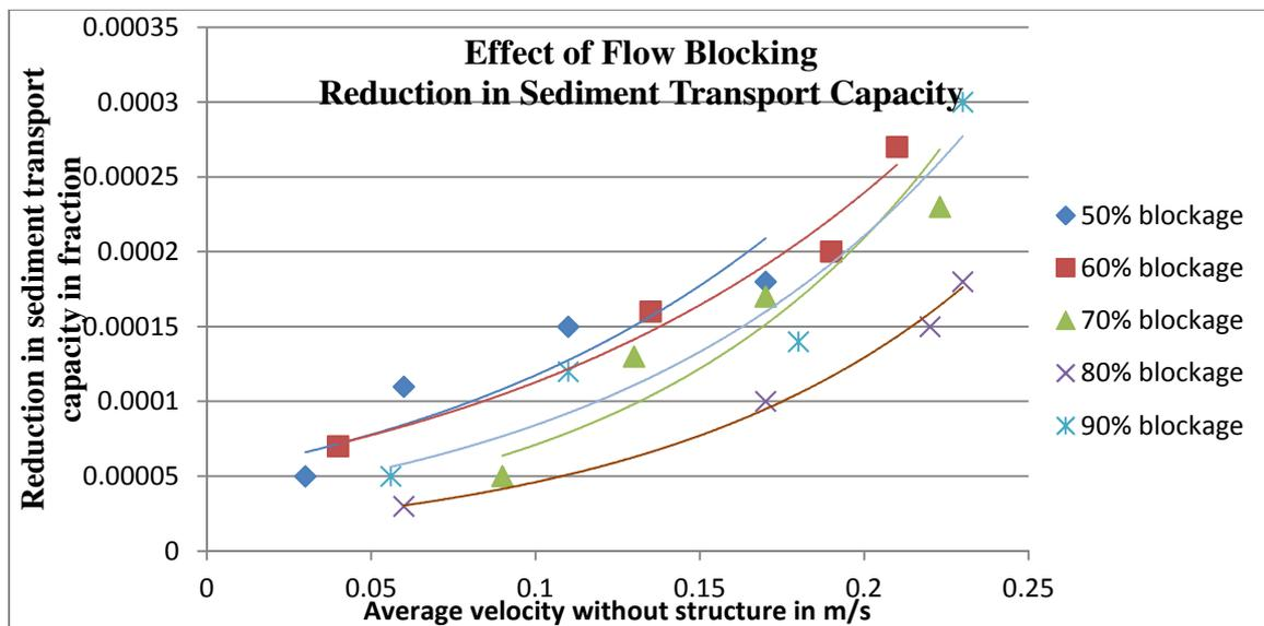
Figure 6 Graph shows effect reduction in sediment transport capacity
