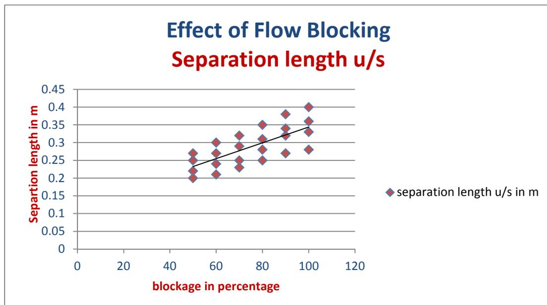
**Figure 1** Graph showing separation length on upstream side vs blockage in %
