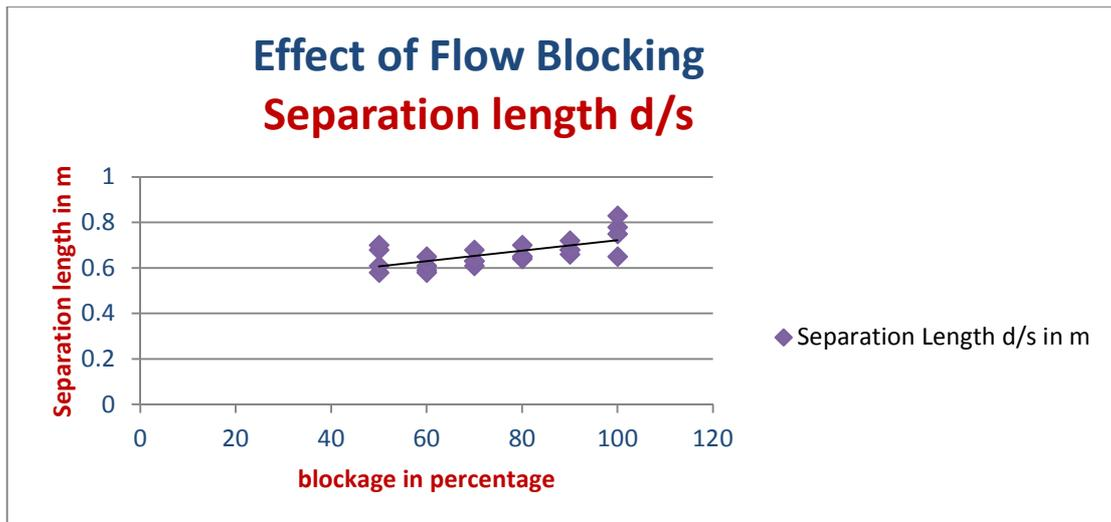
Figure 2 Graph showing separation length on downstream side vs blockage in %
