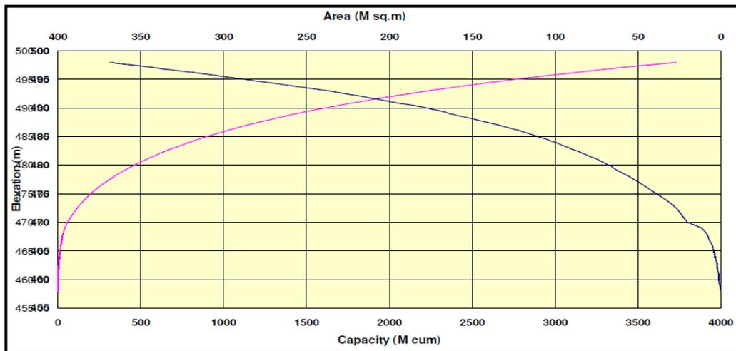
Fig. 2: Elevation-Area-Capacity Curve for Ujjani Reservoir for the Year 1977 (Original)
