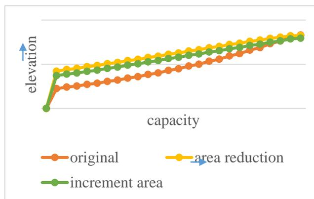
As it is seen in figure 3, the volume-height graph obtained through area reduction method shows better conformance to original values (hydrography).
