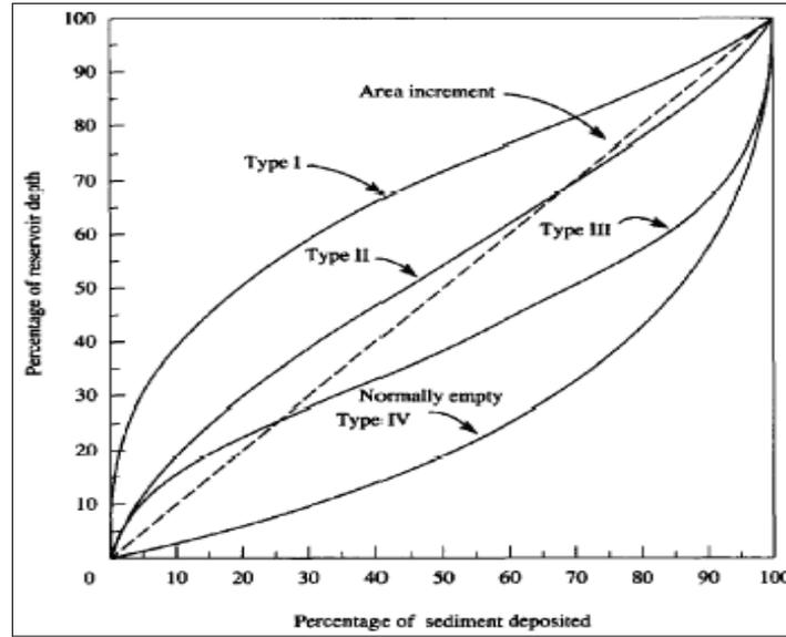
Fig 1: Type curves of reservoirs for area reduction method (modified Strand and Pemberton, 1987).
