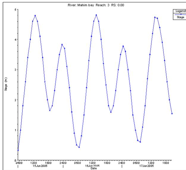
**Figure 6** Three days observed tidal level at Bandra point
