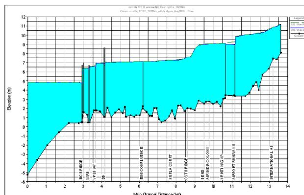
Figure 8 Longitudinal profile of the maximum flood water level along with bed profile for existing condition
