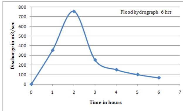
**Figure 5** Typical hydrograph for sub-catchment ‘A<sub>1</sub>’
