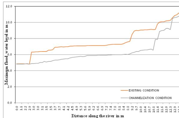
**Figure 10** Comparison of maximum flood water level for existing and channelization condition
