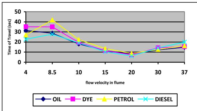
**Graph 2:** Variation of times of travel with varying water flow in flume
