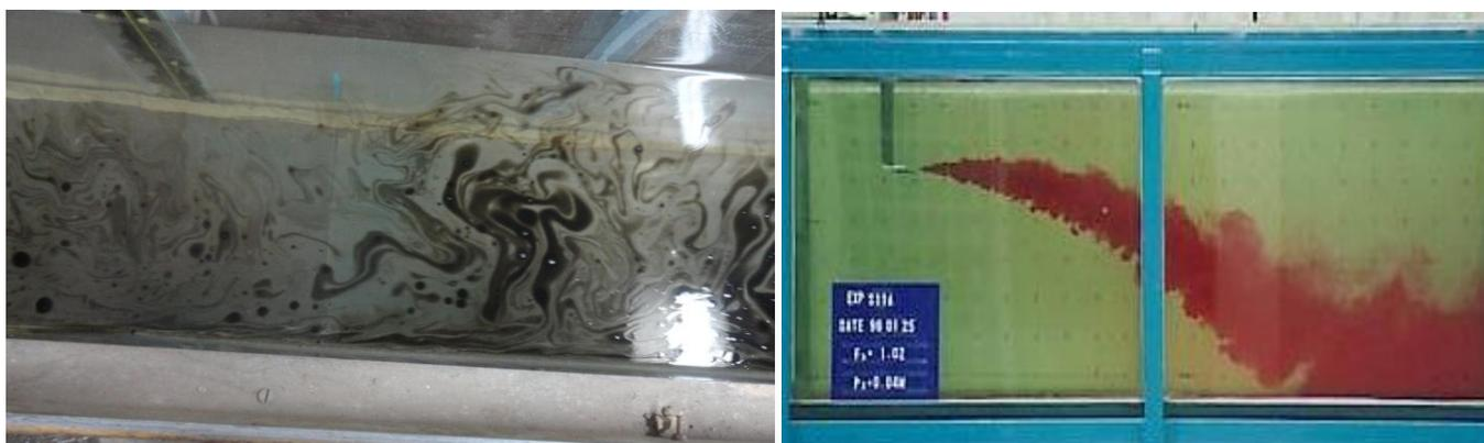
**Fig 2:** Dispersed oil and diffused dye in flume
