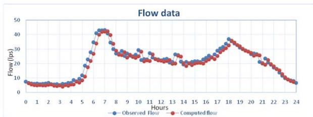
Figure 3: The computed and observed value of inlet meter flow
