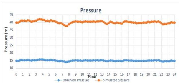
Figure 6: Simulated and observed value of pressure at pressure monitoring point 2 before calibration
