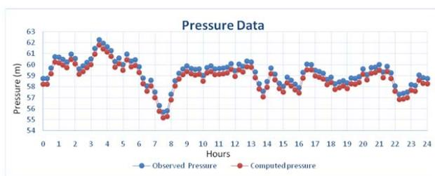
Figure 4: The computed and observed value of pressure data at inlet meter
